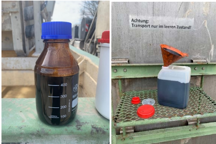
Samples of water free 32 API oil collected from Anshof-3 well flow test. Source ADX
