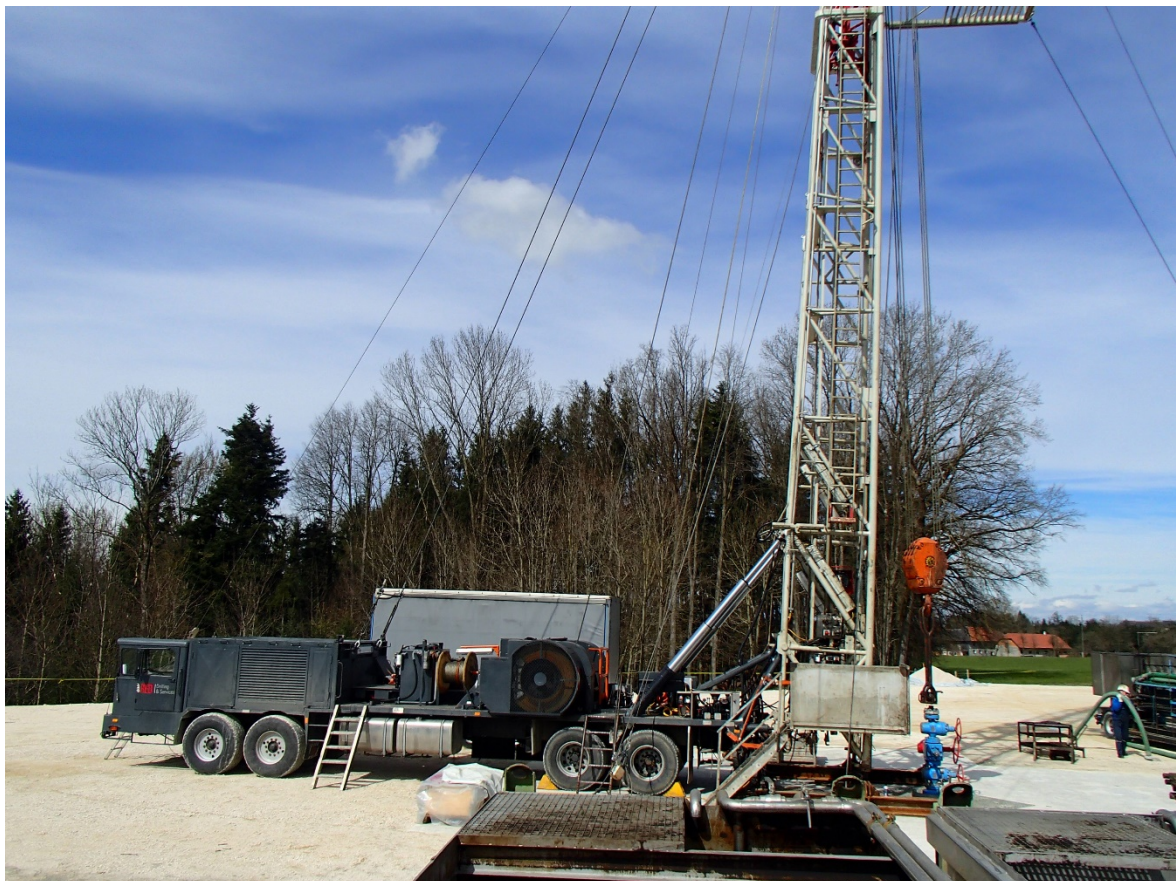
The RED W-101 workover rig set up over Anshof-3 well head in preparation for testing operations. Source ADX
