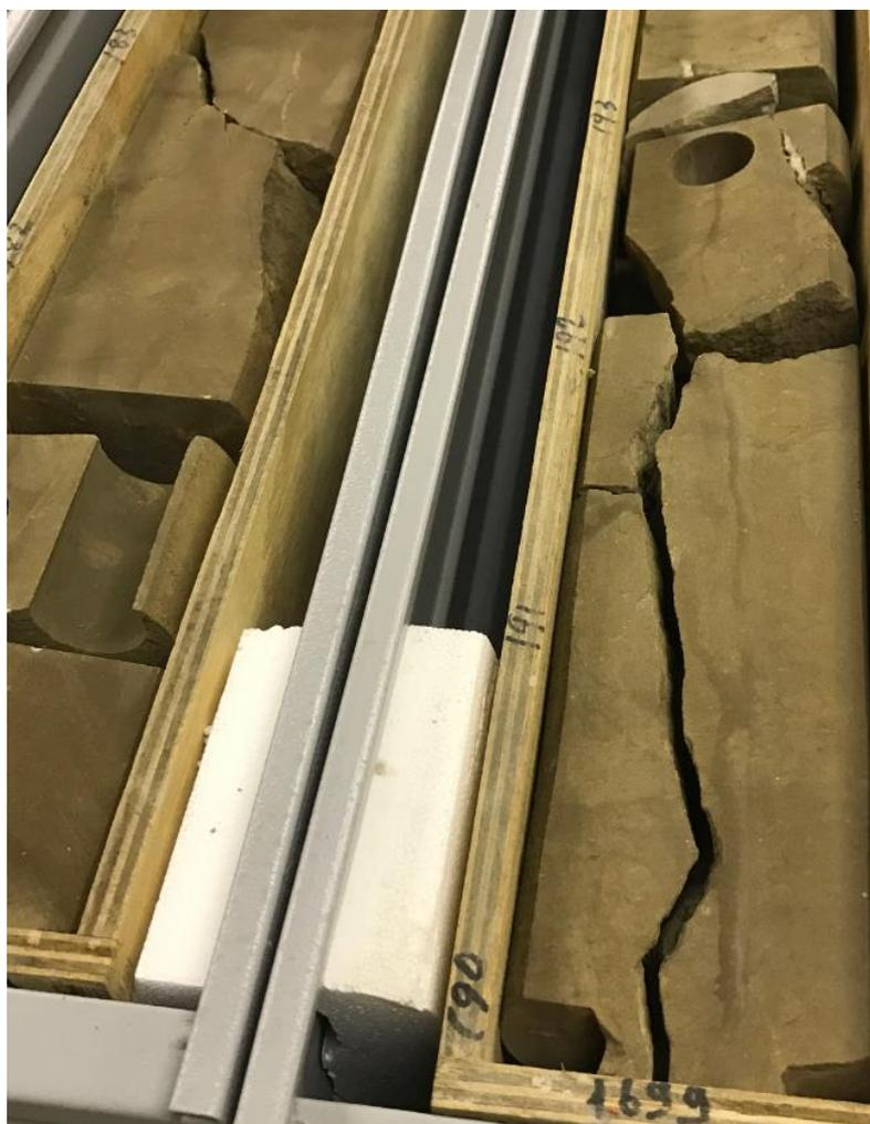
**An example of oil reservoir core from Nilde-6 production well (1699 to 1700 meters MD). Note large scale sub-vertical fractures which facilitated the high flow rates of the Nilde wells. Conjugate geometry suggests well connected fracture system. Brownish color is due to oil staining.**
